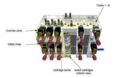
The Heye valve block concept consists of two blocks, on for the blank side and one for the blow side. The operator can directly see what is happening before him, nothing is hidden (other suppliers use one valve block for both sides and have bad or no sight to the other side). In addition, Heye uses a metal cover for the valve blocks, so an accidental release of a valve is excluded.
