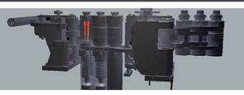
Together with a well-reputed container glass manufacturer Heve is glad to start a project for the implementation of a NNPB lightweight production in China. Start of production is scheduled for autumn this year. The NNPB-process, invented by Heye, makes a thinner and more even wall thickness possible. Weight is reduced and as a consequence, energy and raw material consumption fall as well.
