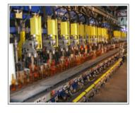
To cover the Australian lightweight market as well, Amcor has decided to build a third furnace with 2 NNPB production lines. The new NNPB production lines have an additional capacity of more than 1 million lightweight bottles a day. Heye
