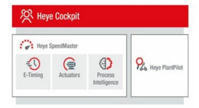
The availability of smart user interfaces for operators has become especially important, as production employees with comprehensive process knowledge are increasingly difficult to find. The Heye Cockpit will become the central user access to the Heye SpeedMaster hot end control and process intelligence portfolio. The Heye SpeedMaster consists of three modules: E-timing; motion control (servo and pneumatic actuators) and the process intelligence
