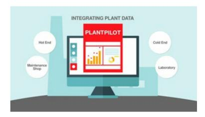
The Heye PlantPilot is the cornerstone in the field of data integration in the glass plant. By using internet-based technology, different machines or modules can be connected to manage the plant. Data integration between hot end and cold end helps especially to gain time. Via the Heye Cockpit, the hot end operator has a perfect overview of the defect situation on the different cavities.
