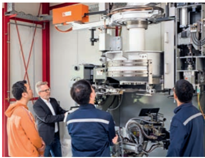
Customer information: how a feeder, plunger, double motor shears and gob distributor work
