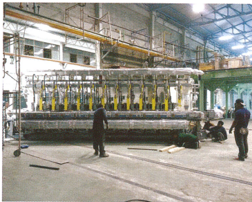
One of the three 12-section triple gob IS machines undergoes installation at L Lighting Glass.
