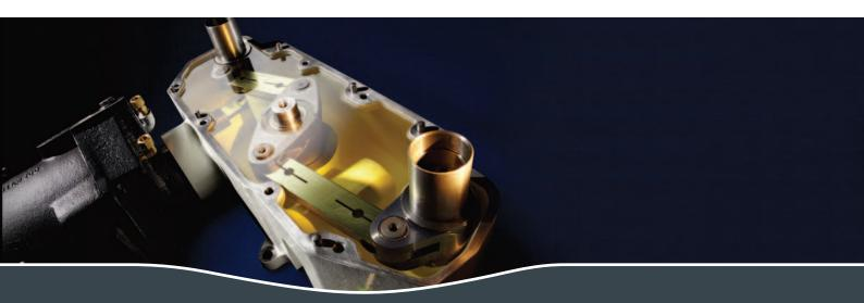
The distribution and quantity of lubrication points in an IS-Machine necessitate the use of a central lubrication system. When this technology was developed, the main priority was sufficient lubrication. At that time, lubricant consumption and system monitoring were not a priority. A reliable level of lubrication was certainly achieved, but the lubricant was not used optimally and faults were difficult to diagnose.
