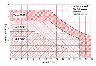
Type 4206: intermittent drive with three servo motors
